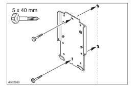
■ Lightly secure retaining plate A into position using 5 x 40 mm screws through the two holes and use the notches to align with the center line.
